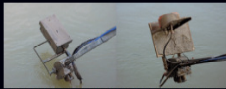
Zweifrequenz Identifikationssonar (DIDSON, links) und Split-Beam-Echolot (FMS, rechts) in der Flussanwendung. Dual-frequency Identification Sonar (DIDSON, left) and Split-beam echosounder (FMS, right) in river application.
